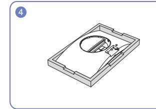
4 Place the protective Styrofoam (cushion) included in the package on the floor and place the product facing down on the Styrofoam, as shown in the image. If Styrofoam is unavailable, use a thick sitting mat.
