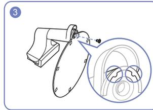
3 Align the stand with the stand neck guide and then turn the screw on the bottom of the stand to fix the stand.
