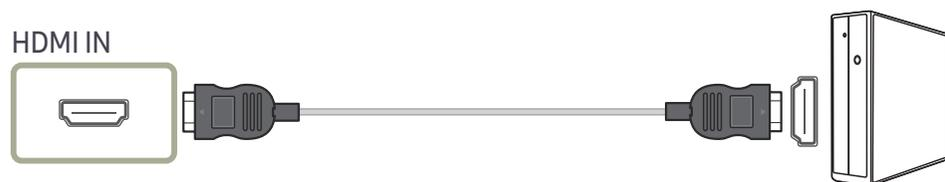
— When connecting an HDMI cable, use the cable that came with the components of the product. If you use an HDMI cable other than provided by Samsung, the image quality may be degraded.
