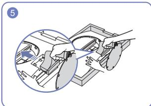
5 Hold the main body of the product with your hand as shown by the figure. Push the assembled stand into the main body in the direction of the arrow as shown in the figure.
