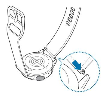
Slide the spring bar inwards and connect the band.
