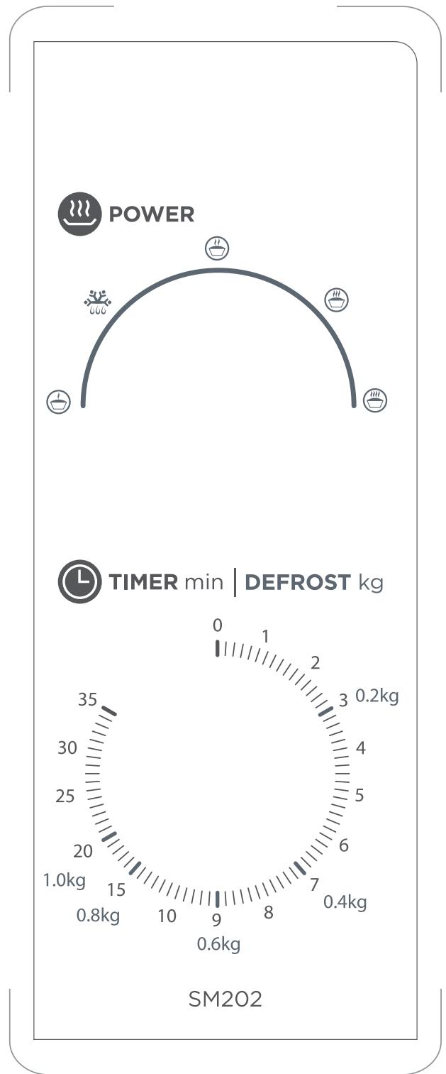
1. Set the desired power level by turning the power and defrost selector knob.
