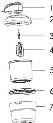
1. Motor unit with I/O power switch
