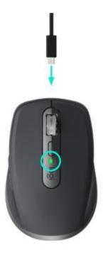
• Connect one end of the provided charging cable to the USB-C port on the mouse and the other end to a USB power source.
