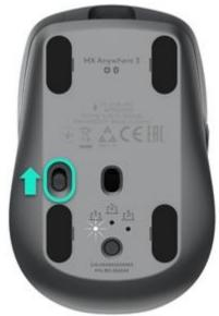
The number 1 LED on the bottom of the mouse should be blinking fast. NOTE: If the LED is not blinking fast, do a long press of three seconds on the Easy-Switch button on the mouse bottom.
