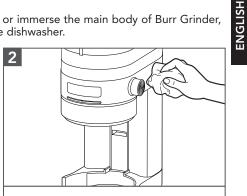
Wipe clean the main body of Burr Grinder with a soft, damp cloth. Dry thoroughly.
