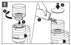
Place the Top hopper onto the machine with the 'Lock icon' facing front. Rotate the Top hopper until it clicks into place.
