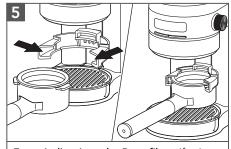
For grinding into the Portafilter: If using a commercial Portafilter (58 mm), insert it into the middle guides of Portafilter holder.
