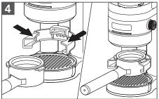
For grinding into the Portafilter: If using a standard residential Portafilter (54 mm), insert it along the top guides of the Portafilter holder.
