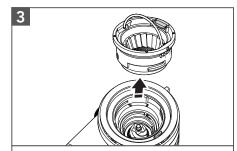
Remove the Top hopper, locate the wire handle on the Upper burr, rotate and lift the handle to remove Upper burr.
