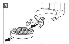
For grinding into a Portafilter: Remove the Grounds catcher tray and then remove the Portafilter holder from its storage location. Insert Portafilter holder into Portafilter holder guide. Replace the Grounds catcher tray.
