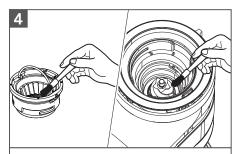
Clean the Upper burr with the cleaning brush. Clean the Lower burr with a brush or use a vacuum cleaner to remove coffee residue.
