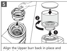
Align the Upper burr back in place and twist clockwise to secure. Replace the Top hopper and the Lid.
