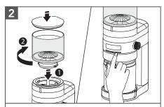
Replace the empty Top hopper and Lid. Press **Start/Stop** ( $\triangleright|\otimes$ ) to run the grinder until empty. Then, unplug the burr grinder.
