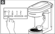
To rinse the Steam Wand, direct the Steam Wand towards the Drip Tray or into a cup. Then, toggle the Mode Button to select Hot Water and press ▶ ⊕ button to start.
