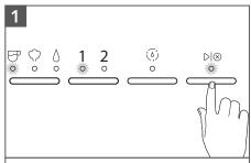
To change pre-programmed Espresso Volume for 1 / 2: Toggle the Mode Button to select Espresso. Select the dose you desire to programme (1 or 2). Press and hold ▶ ⊗ button until desired espresso amount is reached in your cup.
