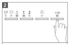
While programming your selected dose, the dose and the **>**1@ button light will blink. Lights will stop blinking when programming is complete.
