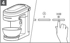
Phase 3: Place the container (~0.5 L) below the Steam Wand. Empty, rinse and refill the Water Tank with fresh water to Max fill line. Replace the Water Tank. Press >1@ button. Start/Cancel (>1@) will blink fast after the third phase is complete. Empty the container.
