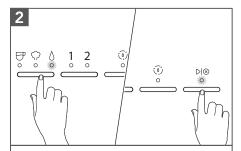
To change pre-programmed Water Hardness: Toggle the Mode Button to Water, Press and hold for 3 seconds. The indicator lights will show the default factory setting or previous saved setting (see Indicator light chart for reference). Toggle the Mode Button between Low-Mid-High to select desired water hardness. To save your selection, press ▶I⊗ button or wait for 10 seconds.
