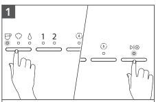
To change pre-programmed Water Temperature: Toggle the Mode Button to select Espresso, press and hold for 3 seconds.
