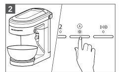
Phase 1: Place a container (~0.5 L) on the Drip Tray below the Group Head. Press the Clean cycle (🕠) button for 3 seconds or until Clean light is solid. Then, press ▶1⊗ button to start first phase of decalcification
