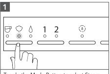
Toggle the Mode Button to select Steam. The machine will automatically start heating, indicated by the flashing Steam light. The Steam light will go solid when machine is ready for steaming.
