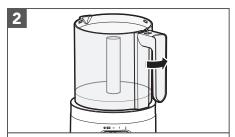
Hold the Handle facing front on the Base. Twist and lock the Bowl in the slots of the Base.
