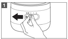
Make sure that the Speed Controller is at "O" position before attaching or removing any parts.
