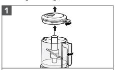
Remove the Lid, Multipurpose Blade, and Drive Adapter. Hold the Base steady. Twist and lift the Bowl to unlock from the Base.
