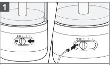
First, slide the Speed Controller to "O". Then, insert the Charger Adapter Pin into the Charging Port.
