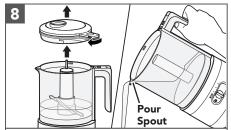
Once processing is complete, remove the Lid, Drive Adapter, and Multipurpose Blade to use the Pour Spout.
