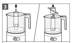
Rotate and lower the Drive Adapter and then Multipurpose Blade or optional Whisking Accessory in the centre of the Bowl until it rests at the bottom.
