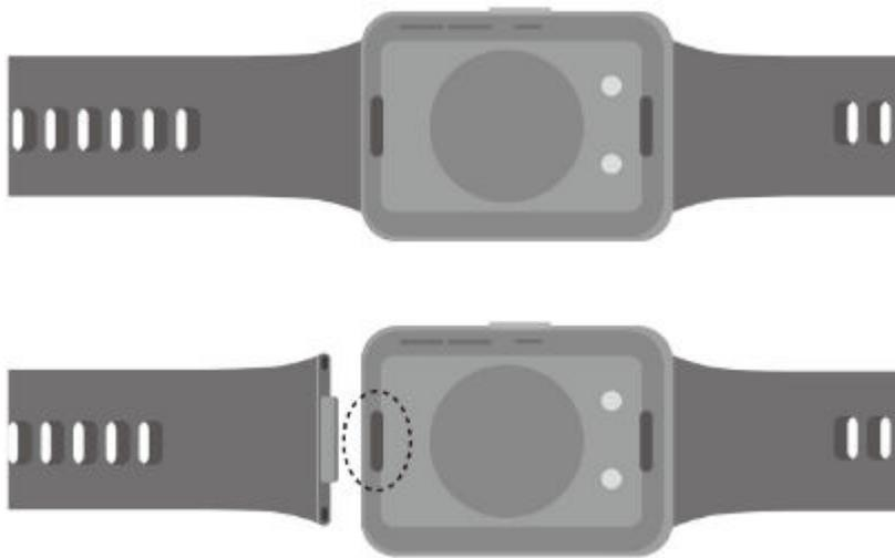
Remove the strap: Press the superfit button on each end of the watch body to separate the strap from the watch body.
