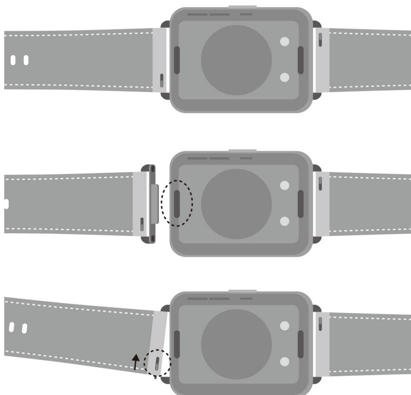
Remove the links: Press the superfit button on each end of the watch body to separate the links from the watch body.
