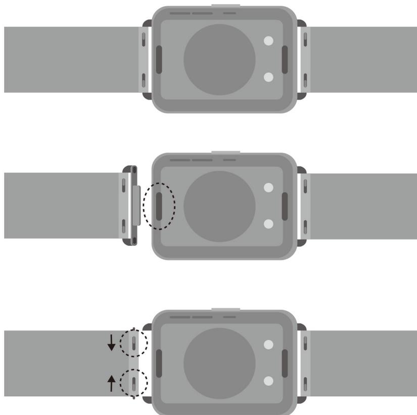
Remove the links: Press the superfit button on each end of the watch body to separate the links from the watch body.
