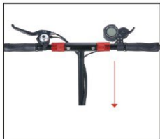
Step 4: Pull downward the T handle bar
