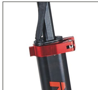
Step4: Fasten the nut and buckle (make sure the stem fixed well)
