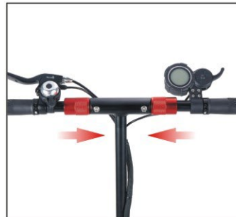
Step2: Extend the T handle bar and fasten the red rods
