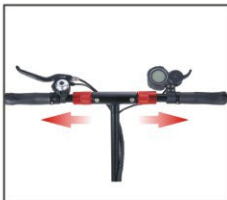
Step 2: Loose the red rods and fold the T handle bar
