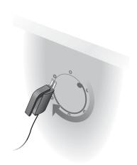
Use a half-round file or wood rasp to smooth out any roughness in the speaker hole you have cut.
