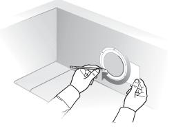
Drill a starter hole that is large enough for your sabre saw blade. Be sure to drill inside and close to the line you have marked.
