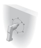
Using the sabre saw, cut the hole for the speaker, carefully staying just inside the line. Take your time; you want a smooth edged circular hole.
