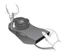
**A CAUTION:** Acoustic performance is reduced if the hole is larger than 1/8 inch (.32 cm) in diameter.
