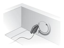
Use a half-round file or wood rasp to smooth out any roughness in the hole you have cut.
