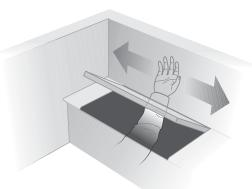
♠ CAUTION: Determine whether any obstacles exist behind the mounting surface. To be certain, contact your boat manufacturer or dealer. Also, be certain that the enclosure will fit within the mounting area before drilling any holes.
