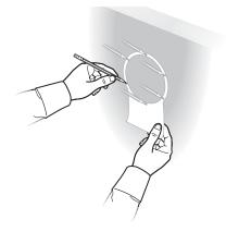
Drill a starter hole that is large enough for your sabre saw blade. Be sure to drill inside and close to the line you have marked.
