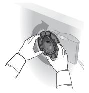
You will need to open *one* of the five marked drain holes because water can enter your 131<sup>™</sup> marine speaker through the ports on the front of the enclosure.
