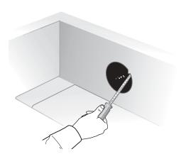
Hold the speaker enclosure up to the hole from behind the bulkhead and find the best position for the extended portion of the enclosure. Be sure the enclosure is hidden behind the bulkhead. If the enclosure does not fit, use the file or rasp to enlarge the hole.
