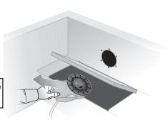
11 Drill the marked holes using a 1/8 inch (.32 cm) bit. Use a center punch to make a slight indentation for your drill bit. This will keep the drill bit from "walking" away from the mark you have made.
