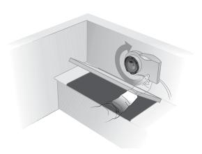
Place the mounting flange so that it interlocks with the enclosure and is flush with the mounting surface.
