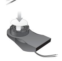
Replace the enclosure behind the bulk head and place the mounting flange so that it interlocks with the enclosure and lines up with the drilled holes. Attach the flange to the mounting surface using six screws
