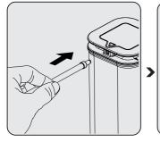
Insert the connection milk tube to the rubber outside the lid. (Open the inlet cover.)
