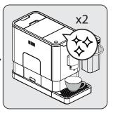
Connect the milk froth system to the machine. Touch the button twice. The button light goes on during the preparation. Press the button once to stop frothing.
