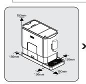
Choose a safe and stable surface with an easily reachable power supply and allow minimum distance from the sides of the machines.
