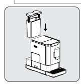
Place the water tank back by using the lid as the handle.
