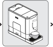
Place a cup under the coffee spout and adjust the height of the spout the fit the cup.
