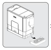
Pull the external drip tray out of the machine.
