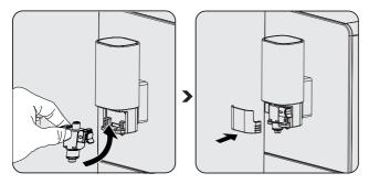
Insert the milk frother to the slot of machine.
