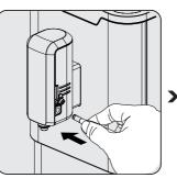
Insert the milk tube connector to the dispensing spout milk frother inlet.
