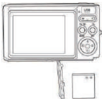
Install lithium battery
