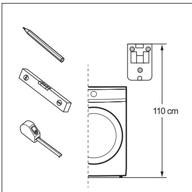
**i** Check where your point of drainage is before positioning the wall support. Filter is equipped with one drainage pipe with length of 100 cm.
