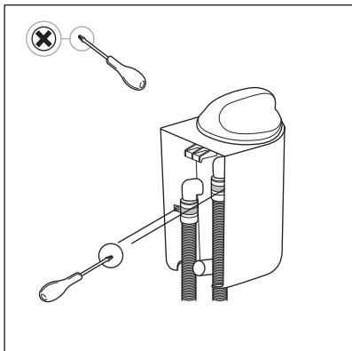
**i** When using the screwdriver, be careful not to damage the filter body or the hoses.
