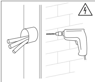
**3. Drill the holes into the wall and place the anchors.**
