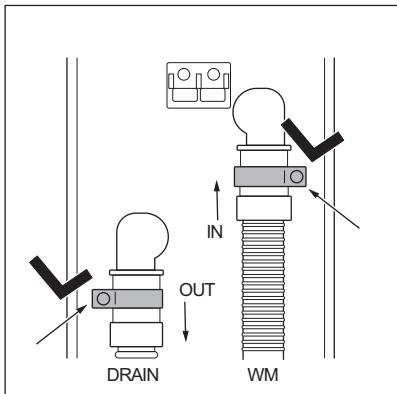
**6. Tighten the collars using the screwdriver.**
