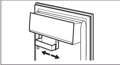
This model is equipped with a variable storage box which can be moved sideways.
