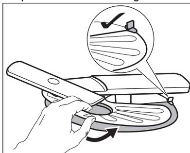
7. Reassemble the filters (B) and (C).
