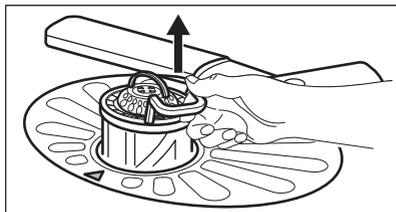
2. Remove the filter (C) out of filter (B).
