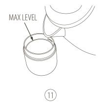
Add boiling water into the water tank. Stop pouring before reaching the step.
