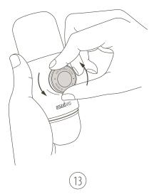
Unlock the piston from its travel position by rotating it to the left.
