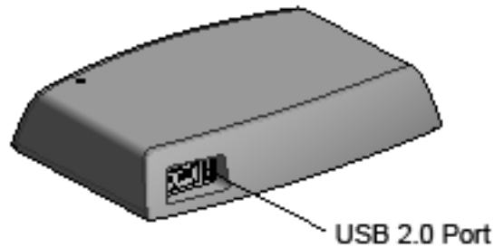
Figure 10: Location of the USB 2.0 Port on Seagate Central
