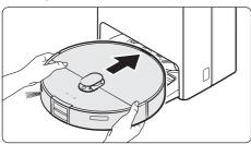
Move the Jet Bot Combo manually onto the Clean Station to recharge.
