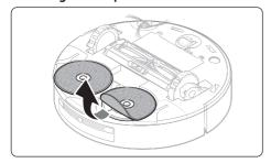
Detach the Mops attached to the bottom of the Jet Bot Combo.
