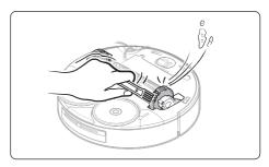
2. Clean the Driving Wheels using the Cleaning Tool.
