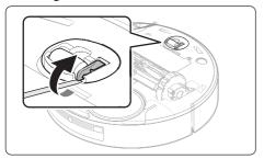
1. Use a flat-head screwdriver to lift the Roller's Release Lever as shown in the figure.
