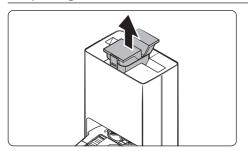
1. Detach the Clean Water Tank from the Clean Station by pulling the handle on the top.
