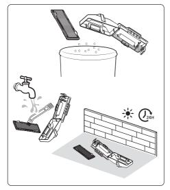
Remove the dust from both the Pre-motor Filter and the Dustbin. Clean them with water and dry both completely in the shade.
