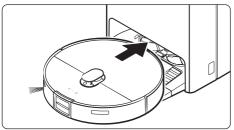
The Jet Bot Combo automatically returns to the Clean Station to recharge when it completes cleaning or when the battery is low.
