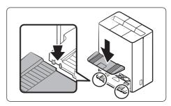
4. Assemble the Base Plate to the Clean Station.
