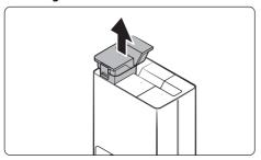
1. Detach the Waste Water Tank from the Clean Station by pulling the handle on the top.
