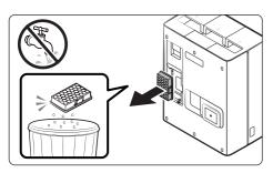
2. Detach the Fine Dust Filter and shake out the dust.
