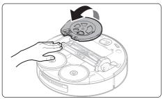
1. Lift the Spin Brush's protective cover in the direction of the arrow as shown in the figure.
