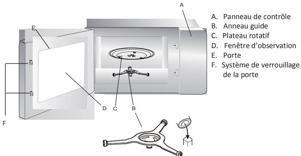
**Plateau rotatif****Connecteur (sous le plateau)**
