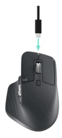
Connect one end of the provided charging cable to the USB-C port on the mouse and the other end to a USB power source.
