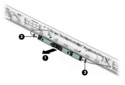
4. To remove the infrared (IR) camera/microphone module:
