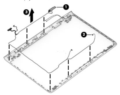
**8.** If replacing the display enclosure, be sure that the subcomponents (including the camera/microphone module, the antenna receivers, and all associated cables and hardware) are transferred to the new enclosure.
