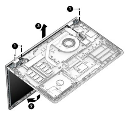
If it is necessary to replace any of the display assembly subcomponents:
