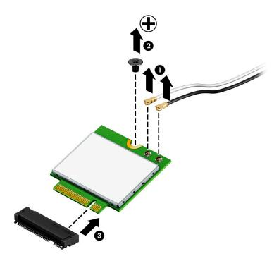
NOTE: If the WLAN antennas are not connected to the terminals on the WLAN module, the protective sleeves must be installed on the antenna connectors, as shown in the following illustration.
