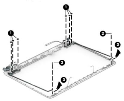
6. To remove the wireless antennas and cables, peel the left(1) and right (2) antennas off the display enclosure, and then remove the antennas and cables from the display enclosure (2).
