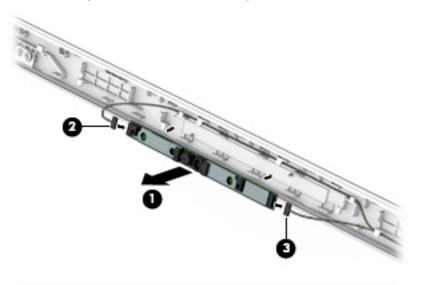
3. To remove the infrared (IR) camera/microphone module:
