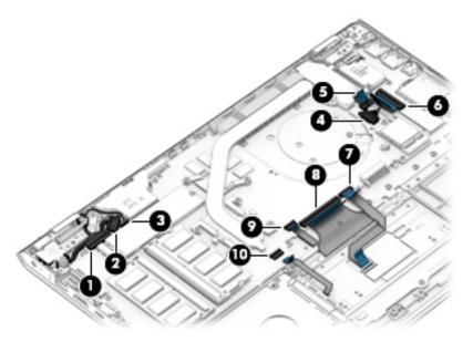
Remove the four Phillips PM2.0×5.0 screws (1) that secure the system board to the computer.
