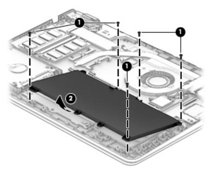
Reverse this procedure to install the battery.
