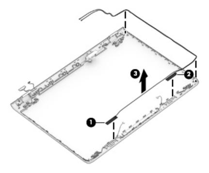
7. To remove the display/camera cable, disconnect the cable from the board at the bottom of the display (1) and the camera at the top of the display (2), and then remove the cable from the clips built into the side of the display enclosure (3).
