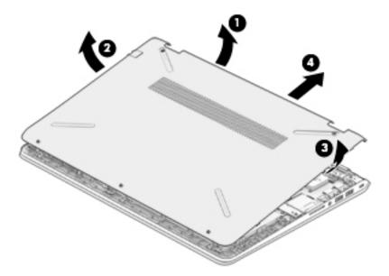
Reverse this procedure to install the bottom cover.
