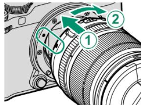
! • When attaching lenses, ensure that dust or other foreign matter does not enter the camera.
