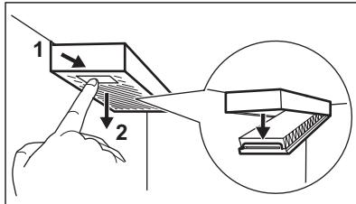
2. Remove the used air filter.
