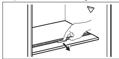
To remove the humidity control device, open the drawer below the glass shelf and pull out the cover.
