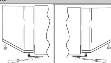
Retire as tampas (A) e (B), desaperte os parafusos e remova parcialmente o painel.
