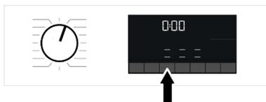
Select the desired auxiliary functions before starting the programme. Whenever a programme is selected, icons of the auxiliary function symbol that is selected together with it illuminates.
