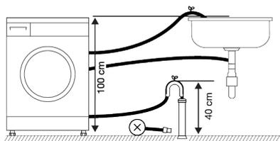
4. To prevent the waste water to go back into the product again and to ensure easy drainage, do not immerse the end of the hose into the waste water or do not insert it into the drain for more than 15 cm. If it is too long, cut it short.
