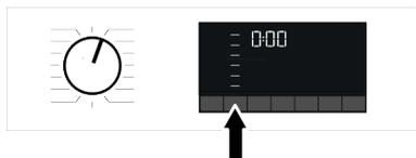
Whenever a new programme is selected, the recommended spin speed of the selected programme is displayed on the Spin Speed indicator. It is possible that the recommended spin speed value is not the maximum spin speed that can be selected for the current programme.
