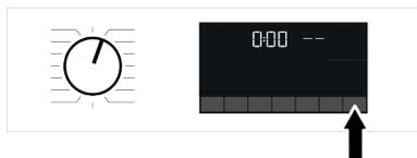
If the water level in the machine is not suitable when you press Start/Pause button, the door lock cannot be deactivated and the door lock icon on the display remains on.
