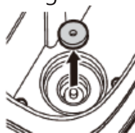
Filtering sponge (side of clean water/solution tank)
