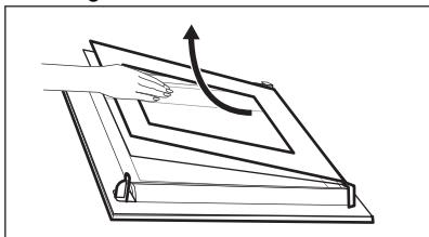
10. Clean the glass panel with water and soap. Dry the glass panel carefully. Do not clean the glass panels in the dishwasher.
